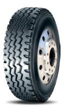
a) Specially designed for steer & trailer axle for on highway application
