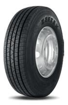
a) Unique tread design with zigzag tread grooves provides good grip and also offers resistance against irregular wear
