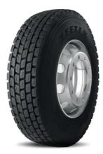
a) Drive Axle Pattern meant for both on/off road applications
