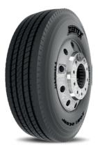
a) 5 rib special design for even distribution of contact pressure and driving stability.
